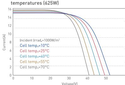
Current and voltage curves/power voltage curves at different irradiance (625W)
